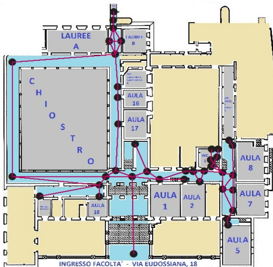
Figure 5.2: The complete routing graph built on the 2D map of the ground floor.
