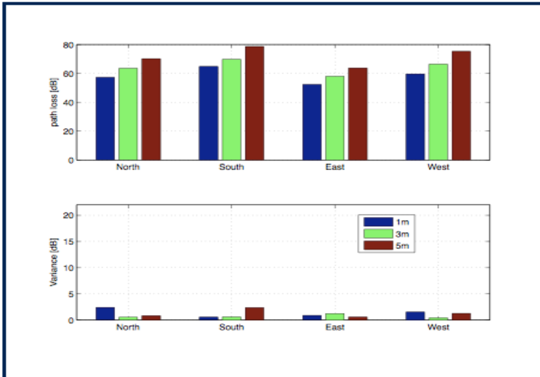
Figure 2.2 Histograms of average path loss and variance (Without user; 1m, 3m, 5m distance from the AP) [ref_Carla]
